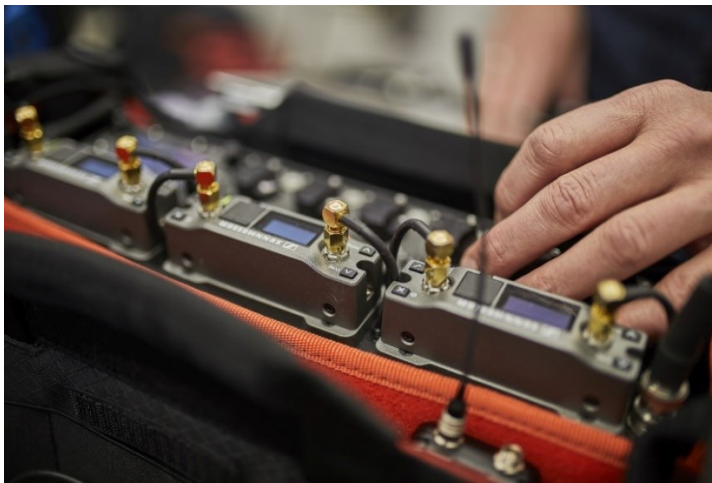
The EK 6042 camera receiver works with analogue and digital Sennheiser transmitters
